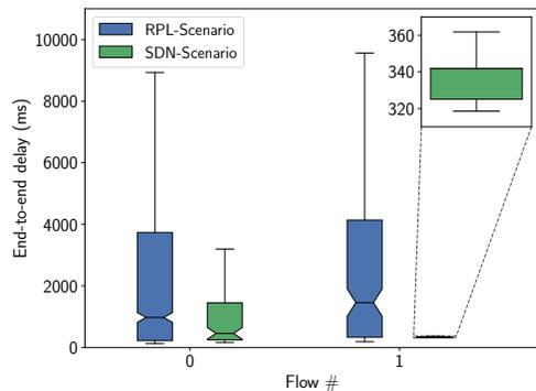
Fig. 7: Delay and jitter of flows in the intermittent interference re-routing scenario (Section V-C). Compares a SDN scenario against a RPL scenario with no SDN. In the SDN scenario,  $\mu$ SDN is configured to reroute flow  $F_1$  around the interference. The achieved reduction in delay and jitter can be seen in the highlighted area of the figure.
